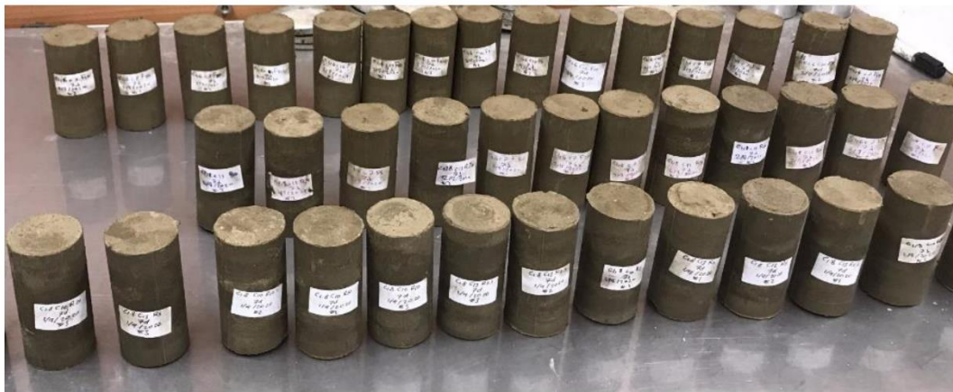
Figure 3.3. Tire-Cement stabilized lightly compacted clay specimens before curing.
